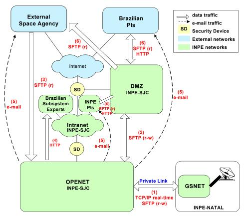
Figure 2. Data Communication for Network Components
